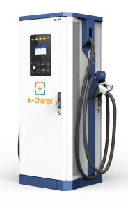
The ICE All-in-One DC Fast Chargers can be flexible configured to up to 180kW of charging power. The EVSE can be used simultaneously (load sharing between both connectors) or sequentially (first in gets full power until charging session ends) depending on the needs of the use case and come with CCS1 and/or CHAdeMO cable types.
