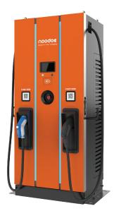
The Noodoe EV Exceed DC series is your ticket to the fastest, most innovative chargers available. This series is a modular, upgradable 90-180 kW charging system with an internal structure that allows for replacing or adding internal 30kW power modules. The Noodoe EV DC Exceed series supports true simultaneous charging and is compatible with all-electric vehicles with CHAdeMO and CCS connectors.
