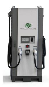
Tellus 120kW Charger adopts innovative design with modular construction. The charger can be configured onsite to deliver either 1 x 120kW or 2 x 60kW (simultaneous charging). It provides wider voltage range from 150VDC - 750VDC providing compatibility to present and future generation EVs. It comes with a Credit Card reader, RFID reader, touch screen interface and is compatible with OCPP standard.
