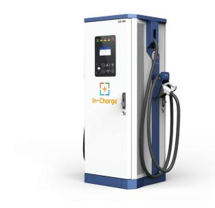
The ICE All-in-One DC Fast Chargers can be flexible configured to up to 180kW of charging power. The EVSE can be used simultaneously (load sharing between both connectors) or sequentially (first in gets full power until charging session ends) depending on the needs of the use case and come with CCS1 and/or CHAdeMO cable types.
