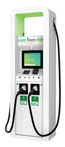
This high-powered charging system is able to charge both today's and the next generation of EVs with a wide voltage range of 150 - 920 VDC. It can charge vehicles at up to 200A for CHAdeMO and 500A for CCS with liquid cooling. Various plug configurations are available; single or dual ports, and a combination of CCS and/or CHAdeMO.
