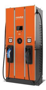
The Noodoe EV Exceed DC series is your ticket to the fastest, most innovative chargers available. This series is a modular, upgradable 120-180 kW charging system with an internal structure that allows for replacing or adding internal 30kW power modules. The Noodoe EV DC Exceed series supports true simultaneous charging and is compatible with all-electric vehicles with CHAdeMO and CCS connectors.
