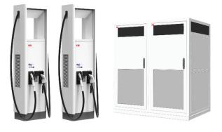
ABB's Terra HP is a modular 175-350 kW charging system supporting 920 VDC vehicles. With Dynamic DC power sharing technology, the Terra HP system is expandable over time. Every Terra HP charge post is equipped with liquid cooled cables for high continuous output power performance, along with an advanced HMI and support for OCPP 1.6 integrations.
